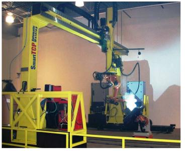
The SmartTCP Automatic Welding Solution automates both the robot programming and weld production. The system is a combination of hardware and software and features a flexible and modular working envelope that allows the manufacturer to weld any weld-able part. The hardware is composed of multiple industrial products from leading industry manufacturers including a gantry system from Gudel Inc., a robot system, external axis motors, control
